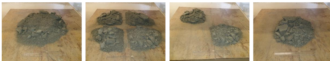
Figure 3: Coning and quartering method: illustration on a sample
